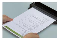
Re-insert the page *without pressing the Scan button* to scan the other side.
