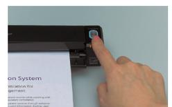
After you finish scanning, press the Scan button to save file.
